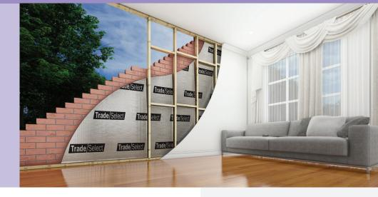
Trade Select<sup>™</sup> Wall Wrap xRS is a Medium Duty, reflective wall wrap designed specifically for use in masonry and brick veneer wall systems to enhance thermal performance.
