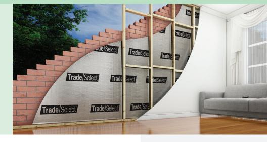
Trade Select™ Wall Wrap Micro-perforated is an Extra Heavy Duty, vapour permeable wall wrap designed for use in brick veneer and drained cavity wall systems to reduce the risk of interstitial condensation in building systems. The reflective foil side provides extra R-value when installed facing an air cavity, and the multi-layer structure provides superior strength, flexibility and durability.
