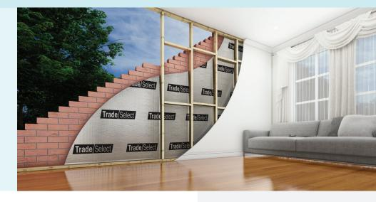
Trade Select<sup>™</sup> Wall Wrap Micro-perforated is a Light Duty, Vapour Permeable wall wrap designed for use in brick veneer and drained cavity wall systems to reduce the risk of interstitial condensation. The reflective foil side provides extra R-value when installed facing an air cavity, and the multi-layer structure provides superior strength, flexibility and durability.
