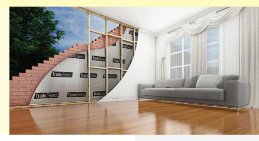
Trade Select<sup>™</sup> Wall Wrap Micro-perforated is a Medium Duty, Vapour Permeable wall wrap designed for use in brick veneer and drained cavity wall systems to reduce the risk of interstitial condensation. The reflective foil side provides extra R-value when installed facing an air cavity, and the multi-layer structure provides superior strength, flexibility and durability.
