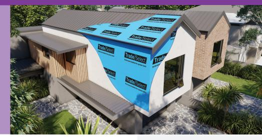
Trade Select™ Sarking xR is a Extra Heavy Duty double-sided radiant barrier, designed for use under metal deck roofs where temperatures can exceed 80°C, and with battened out cladding to create an extra reflective air space for enhanced R-Value. It is an Air and Water Barrier, Class 2 Vapour Barrier product, suitable for use in roof and wall applications.
