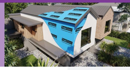
Trade Select™ Sarking xR is a Extra Heavy Duty double-sided radiant barrier, designed for use under metal deck roofs where temperatures can exceed 80°C, and with battened out cladding to create an extra reflective air space for enhanced R-Value. It is an Air and Water Barrier, Class 2 Vapour Barrier product, suitable for use in all roof and wall applications.
