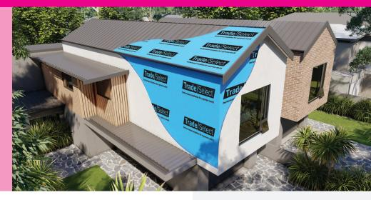
Trade Select™ Sarking xR HD is a Heavy Duty double-sided radiant barrier, designed for use under metal deck roofs where temperatures can exceed 80°C, and with battened out cladding to create an extra reflective air space for enhanced R-value. It is an Air and Water Barrier, Class 2 Vapour Barrier product, suitable for use in all roof and wall applications.
