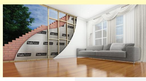
Trade Select™ Wall Wrap Micro-perforated is a Medium Duty, Vapour Permeable wall wrap designed for use in brick veneer and drained cavity wall systems to reduce the risk of interstitial condensation. The reflective foil side provides extra R-value when installed facing an air cavity, and the multi-layer structure provides superior strength, flexibility and durability.
