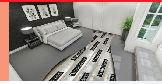
Trade Select "SilverFloor" is a Heavy Duty, vapour permeable floor insulation, designed for use under floors with a sealed air space between flooring and enclosed sub-floor space. Double-sided reflective surfaces provide increased R-value to your floor system. 5 mm weep holes at 400 mm intervals in the membrane structure allow water and water vapour to permeate through, preventing moisture build-up under flooring.
