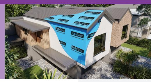
Trade Select<sup>™</sup> Sarking xR is a Extra Heavy Duty double-sided radiant barrier, designed for use under metal deck roofs where temperatures can exceed 80°C, and with battened out cladding to create an extra reflective air space for enhanced R-Value. It is an Air and Water Barrier, Class 2 Vapour Barrier product, suitable for use in all roof and wall applications.
