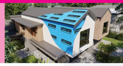
Trade Select<sup>™</sup> Sarking xR HD is a Heavy Duty double-sided radiant barrier, designed for use under metal deck roofs where temperatures can exceed 80°C, and with battened out cladding to create an extra reflective air space for enhanced R-value. It is an Air and Water Barrier, Class 2 Vapour Barrier product, suitable for use in all roof and wall applications.
