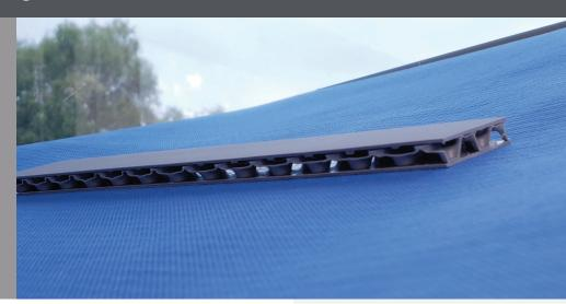
Ametalin Cavity Drainage Battens™ is an innovative triple-layer, high-density polypropylene, self-adhesive, passive open air-flow strip. They are specifically designed to isolate and create ventilation, cavity drainage, and thermal separation in either vertical or horizontal orientation between pliable building membranes and various cladding materials and roofing sheets while providing a hard base to install to.
