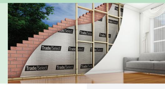
Trade Select<sup>™</sup> Wall Wrap Micro-perforated is an Extra Heavy Duty, vapour permeable wall wrap designed for use in brick veneer and drained cavity wall systems to reduce the risk of interstitial condensation in building systems. The reflective foil side provides extra R-value when installed facing an air cavity, and the multi-layer structure provides superior strength, flexibility and durability.
